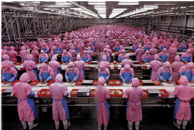
Figure 3. Hand place/ Insert/ Solder Components that have been Kitted and Delivered to Single Operator Stations
