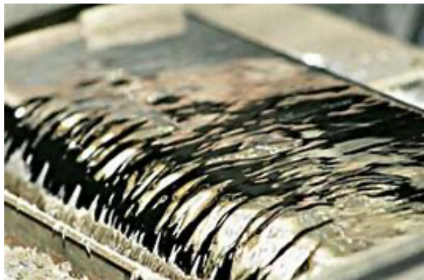
Figure 8. Wave Soldering – The Solder Wave
