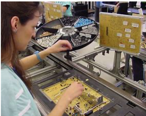
Figure 4. Single Station Build – Manual Labor
